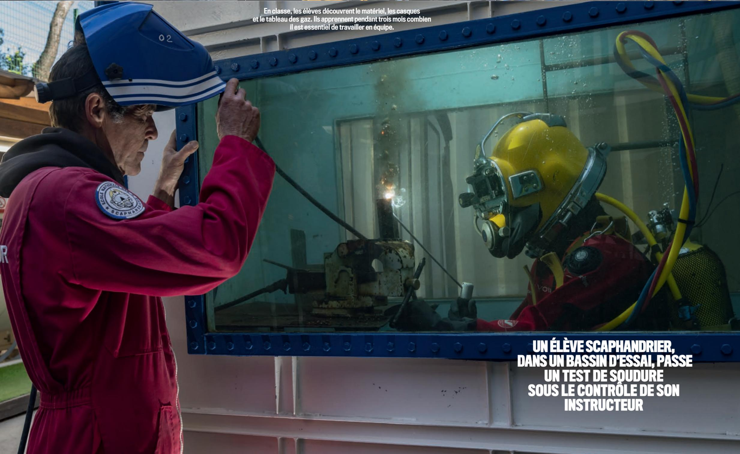
**UN ÉLÈVE SCAPHANDRIER, DANS UN BASSIN D'ESSAI, PASSE UN TEST DE SOUDURE SOUS LE CONTRÔLE DE SON INSTRUCTEUR**
